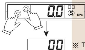
※ The limit of zeroing setting is less than 2%FS
