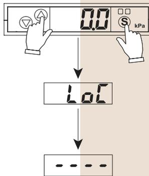
※ Touch button lock: Simultaneously press **△** and **S** for **S** seconds.
